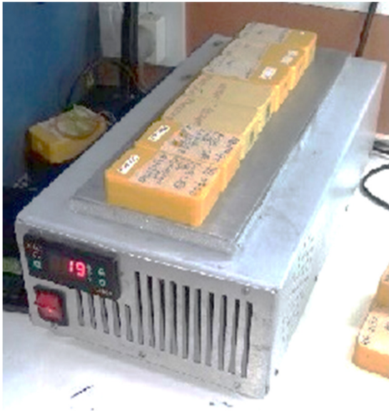
Cooler machine with Aluminum plate on top to cool rubber molds after wax pulling
